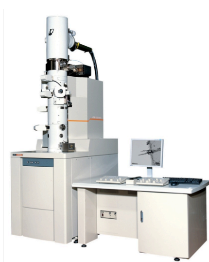
The JOEL JEM-2200FS Energy Filtered Transmission Electron Microscope scheduled for installation in late 2013.
